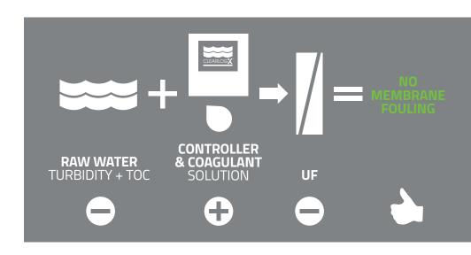
The Clearlogx™ technology optimizes coagulant addition based on the level of turbidity & soluble organic to enhance their removal. The process also controls acid or base feed to regulate the pH. This control technology reduces particles & flocs attraction to the membrane surface and improves the overall treatment process.
